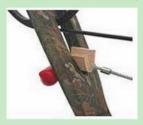
Now turn the screw so the tension is removed from the bowstring. Remove and replace the string if that is what you are doing, then reverse the above. If dismantling the bow, remove the string and then turn the screw until all of the tension is out of the limbs. You might need to fiddle with dimension B if it is too small to remove the string.
